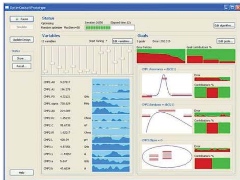
The ADS optimization cockpit provides an interactive environment with multiple optimization variables, interactive tuning and progress controls. Achieve the best performance while gaining design insight of the optimized variables versus the goals.
